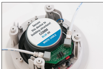
Typical connection of ethernet cables to speaker
