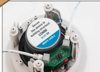
Typical connection of ethernet cables to speaker
