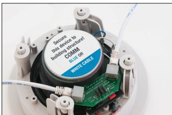
Typical connection of ethernet cables to speaker
